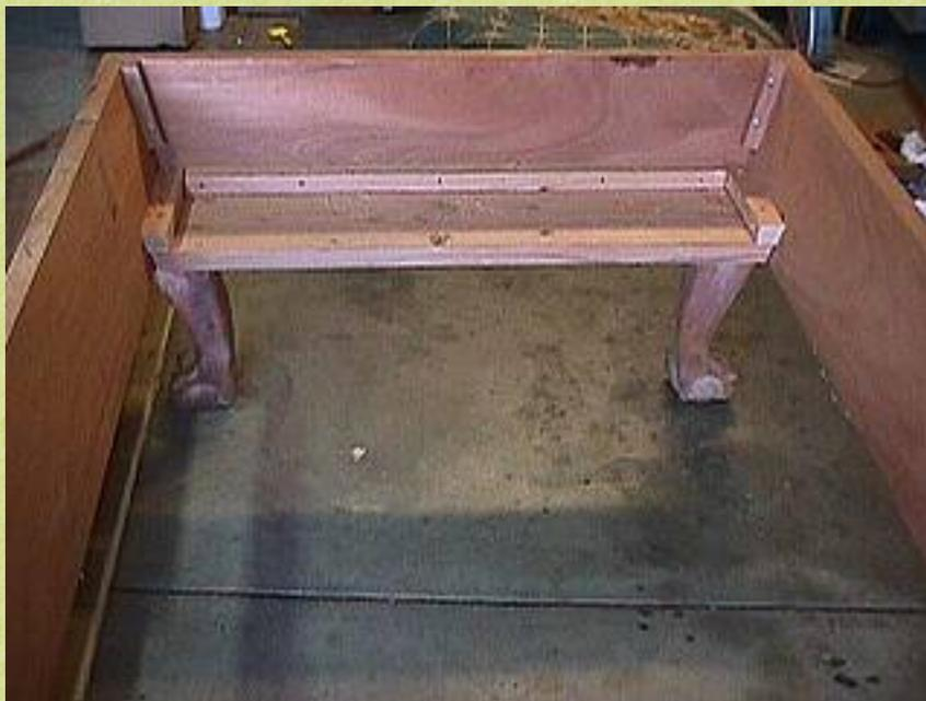
degree bevel at the end then layed one of my support boards in place and glued in the beveled sides. I placed my two 10 inch glue blocks at either end of the support boards and screwed them into place using 2 inch #10 screws. I did the same at the other end. I then layed in the rest of the left over Fir at the end. Cut them with 90 degree ends so they would fit tightly between the other two glue blocks. I ran 2 inch screws in both directions (down and out).
