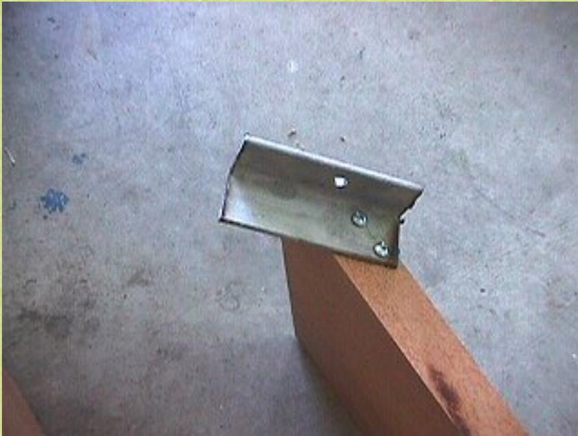
After all the brackets were installed I flipped each board over and ran a 5/8 inch all thread through each matching hole on each bracket.
